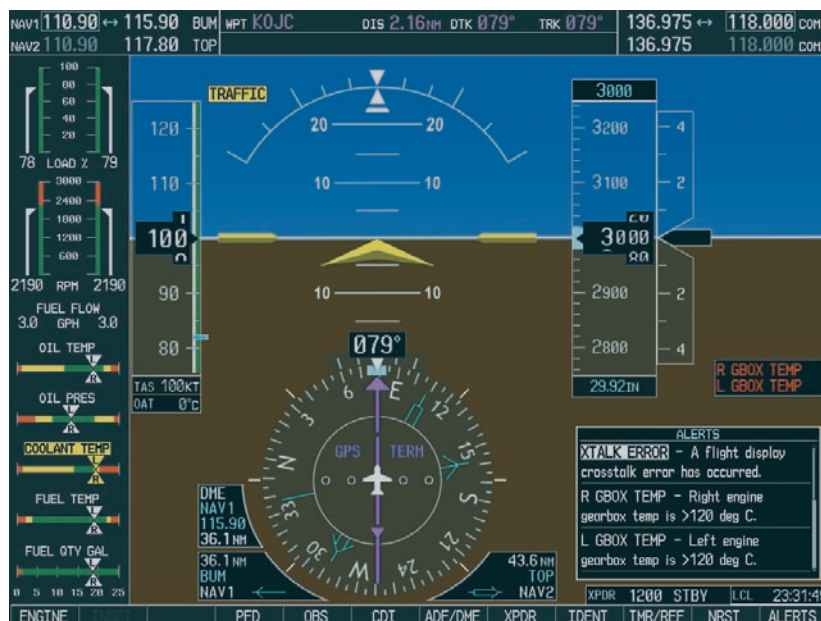
Figure 3.7.1 PFD Reversionary Mode
