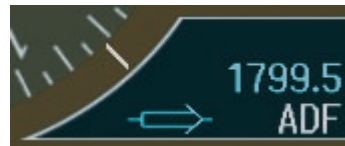
Figure 3.4.24 ADF Selected in BRG2 Information Window
