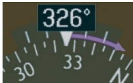
Figure 3.4.18 Turn Rate Indicator and Trend Vector
