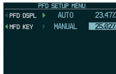
Figure 3.2.1 PFD Setup Menu Window
